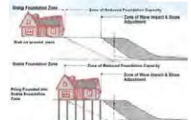
Piling into Stable Foundation Zone – Gosford DCP
