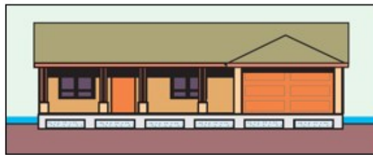
Raising the slab on waffle pods is effective in reducing the possibility of the house being inundated by overland flooding 4
