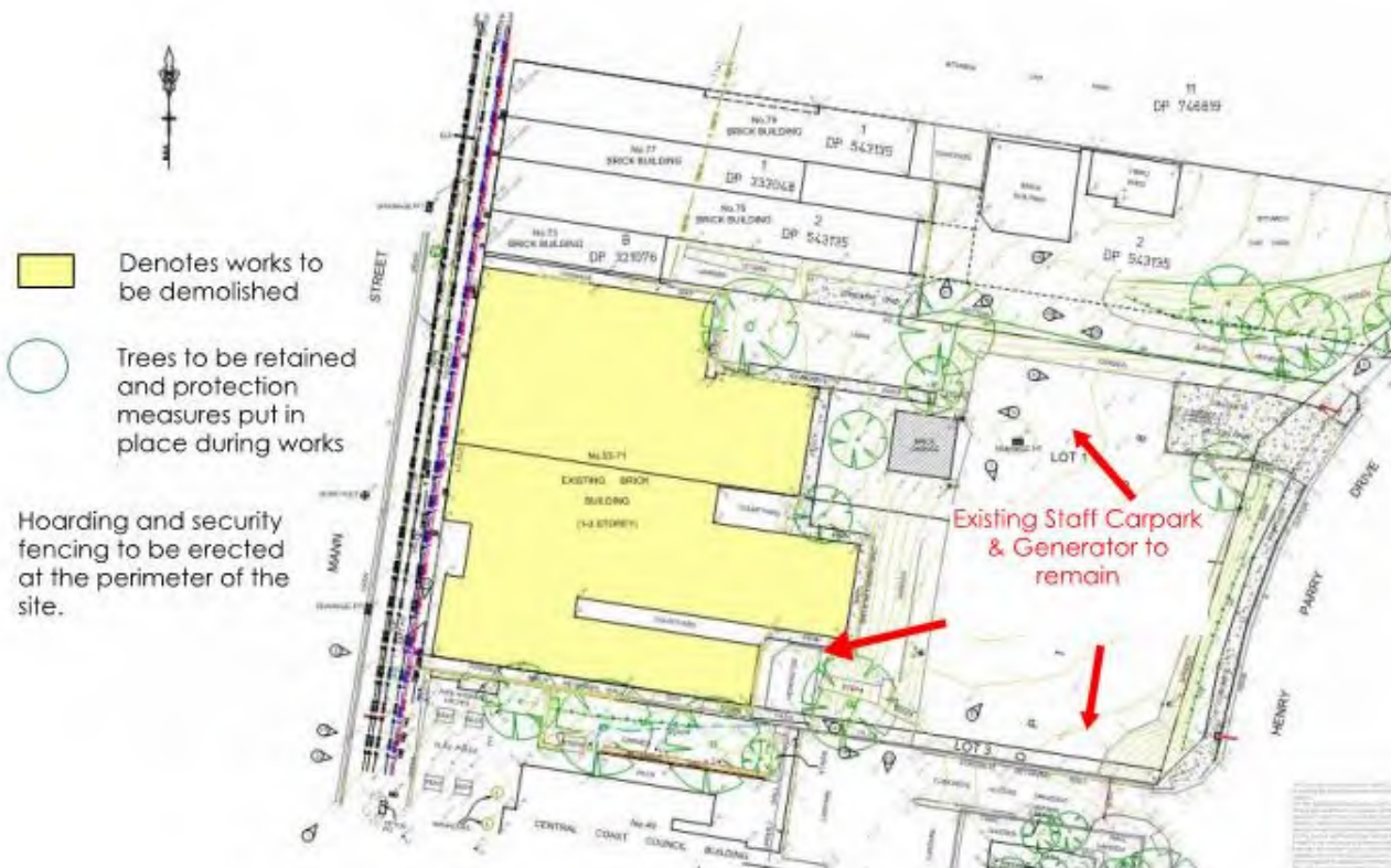
Figure 3: Extract of site/demolition plan
