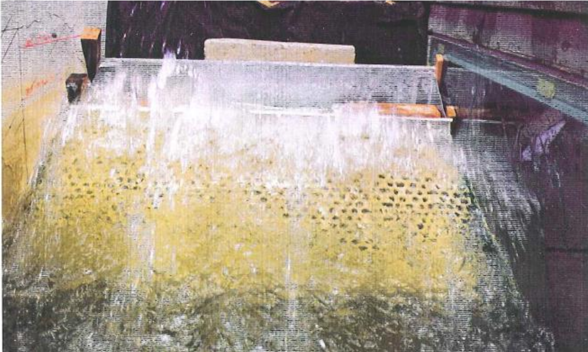
Figure 4.14 Overhead view of wave runoff
