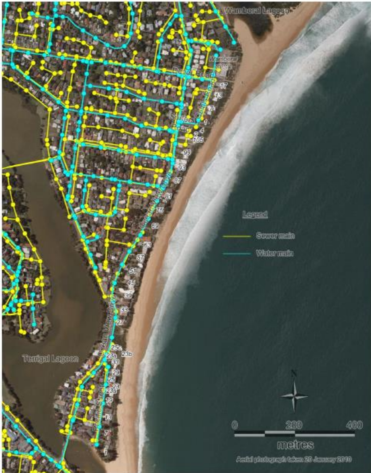
Figure 9.3 Sewer and water infrastructure (WP, 2017, Figure 9)
