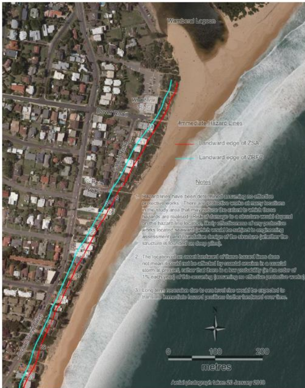
Figure 22: Immediate Coastline Hazard Lines at landward edge of Zone of Slope Adjustment (ZSA) and Zone of Reduced Foundation Capacity (ZRFC) in northern half of study area (ignoring protective works)
