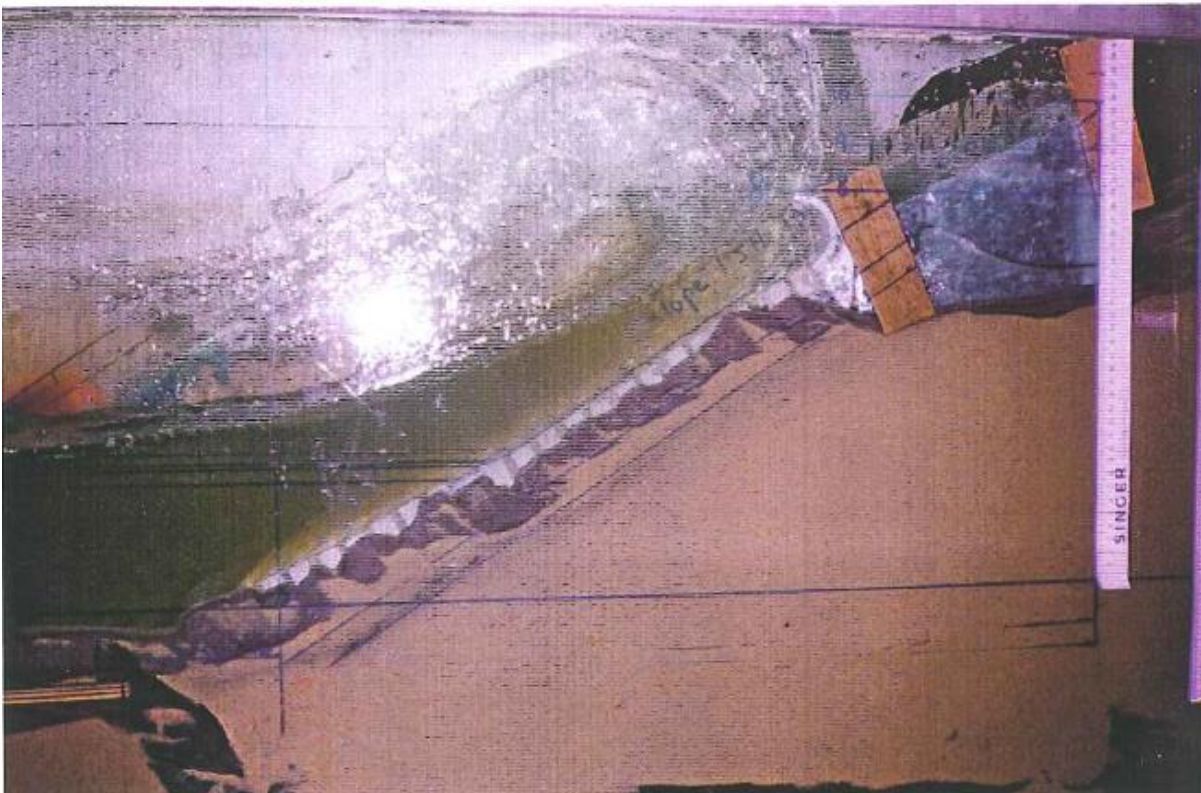
Figure 4.13 Side view of wave runup
