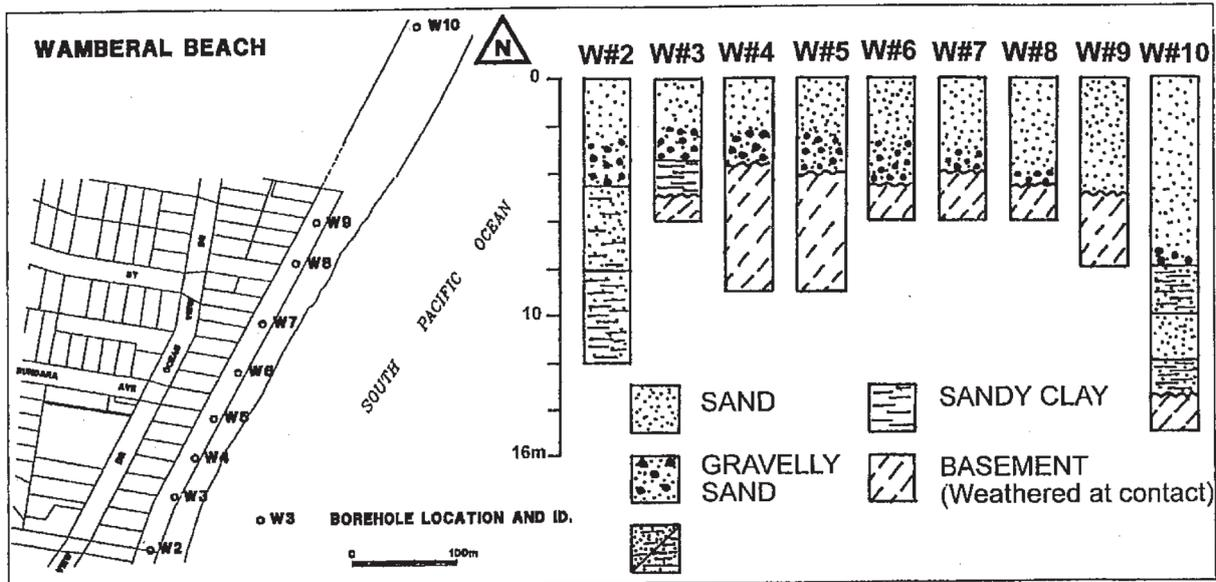
Figure B.4: Wamberal Beach borehole samples from Hudson (1997). Siltstone/claystone unit interpreted as bedrock.
