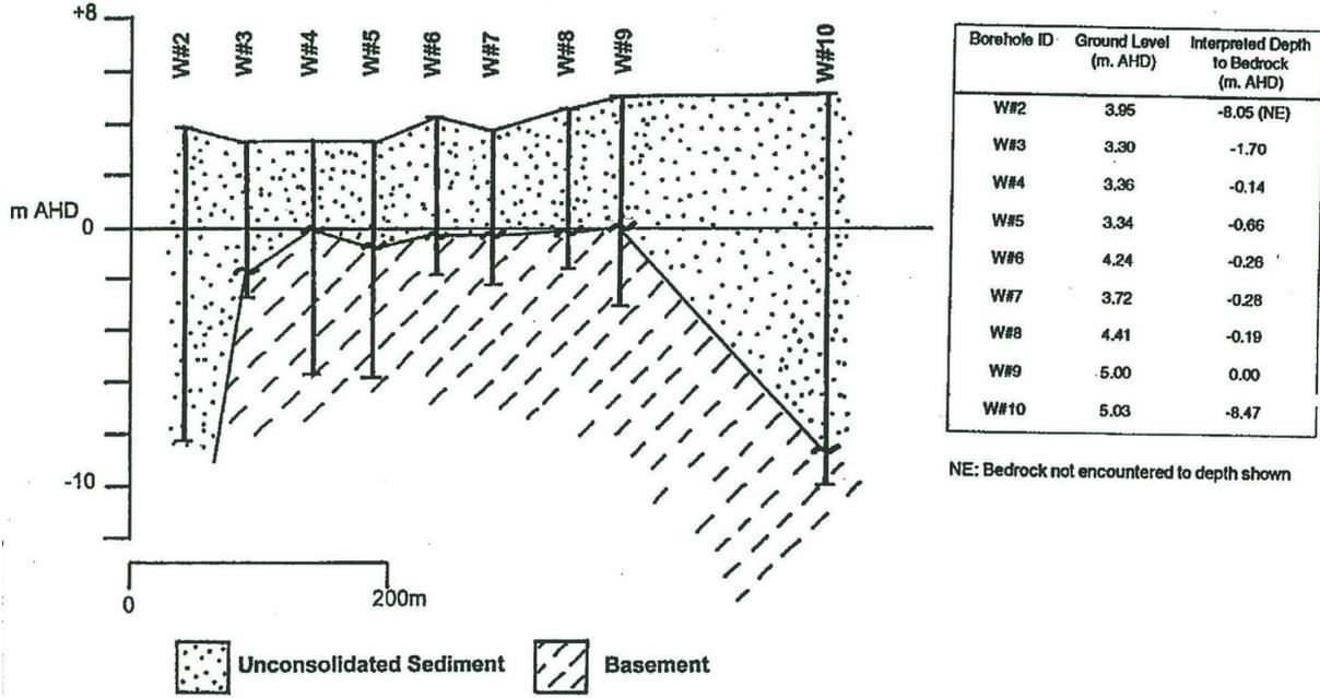
Figure B.5: Wamberal Beach Geological Section from Hudson (1997). Siltstone/claystone unit interpreted as bedrock.
